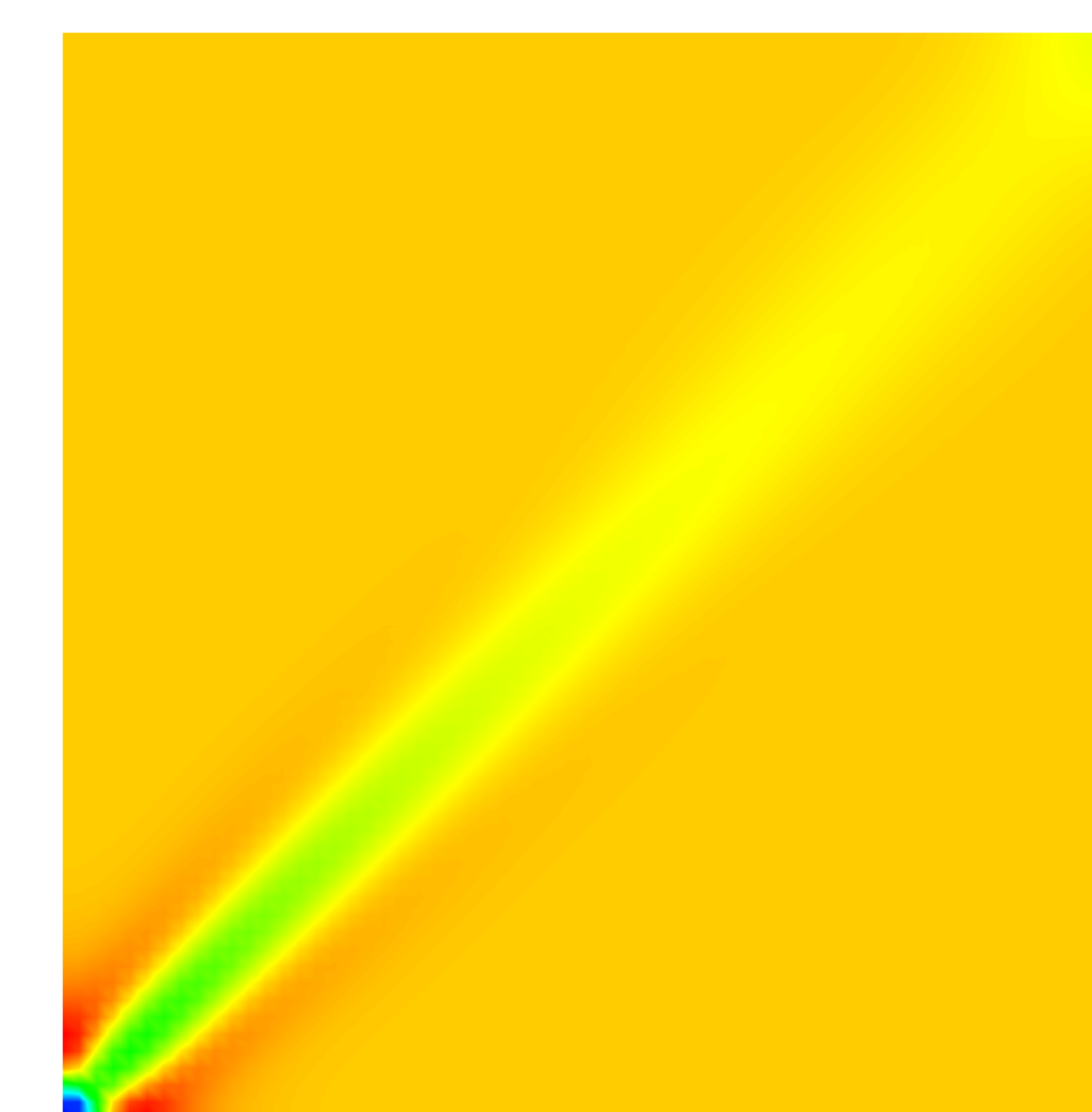
Figure 4: Strain rate invariant for the extension experiment. While this model has a resolution of 64x64 and \tan\phi=0.5 , this result is typical for all resolutions and \phi .
