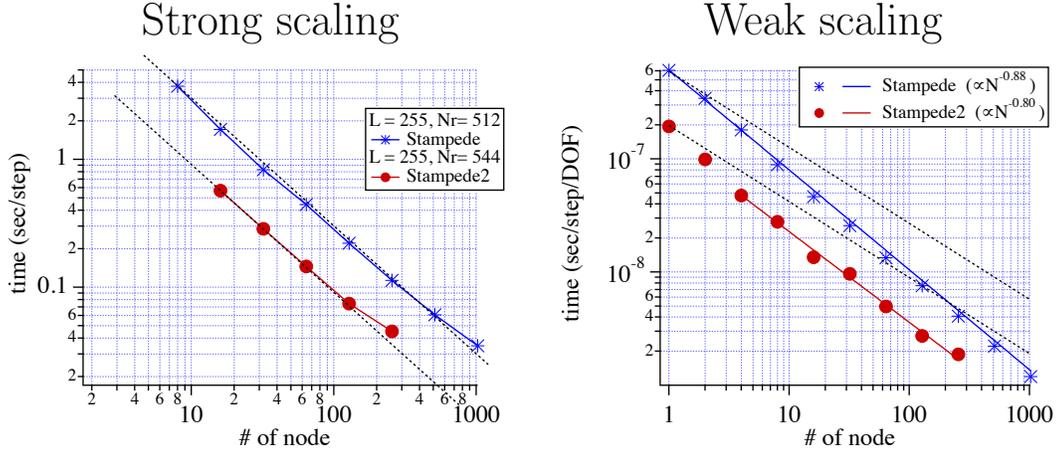
Figure 1: Comparison of performance of Calypso on Stampede2 and Stampede. Strong scaling result is plotted on the left, and weak scaling result is shown in the right. Ideal scaling is plotted by the dotted lines, and fitted results of the weak scaling is shown by solid lines.
