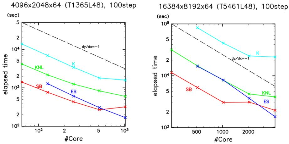
Figure 3: Strong scaling of SPmodel as a function of number of processor core. Results with  $(N_r, l_{max}) = (48, 1365)$  is plotted in the upper panel, and results with  $(N_r, l_{max}) = (48, 5461)$  is plotted in the lower panel. Results on Stampede 2, Stampede, Earth Simulator 3, and K computer are plotted by green, red, blue, and cyan, respectively.
