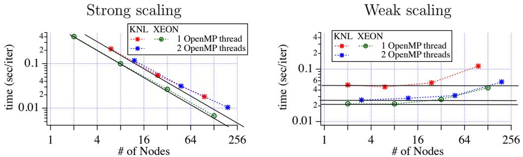
Figure 3: SPECFEM3D\_globe scaling on the TACC Stampede2. Strong scaling results is shown in the left, and weak scaling results are shown in the right. Ideal scaling ( $O(N_{node}^{-1})$  and constant for the strong and weak scaling, respectively) is plotted by solid lines. In the scaling tests for the KNL nodes, 64 of 68 processor cores are used and 1 or 2 OpenMP threads cases are tested.
