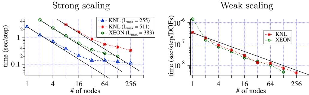
Figure 2: Rayleigh's scaling on the TACC Stampede 2. Strong scaling results is shown in the left, and weak scaling results are shown in the right. Ideal scaling ( $O(N_{node}^{-1})$  and  $O(N_{node}^{-2/3})$  for the strong and weak scaling, respectively) is plotted by solid lines. Rayleigh only uses MPI parallelization, and 64 of 68 processor cores are used in the each KNL node.
